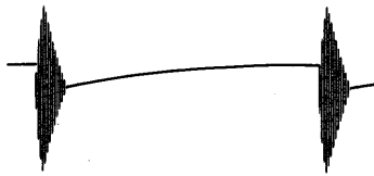
Fig. 5 - Waveform at plate of burst amplifier
